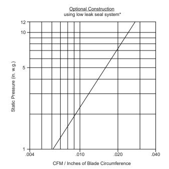
\* Low Leakage seal system consists of: rubber seal bolted to blade, stuffing box with packing gland material, and outboard bearing.
