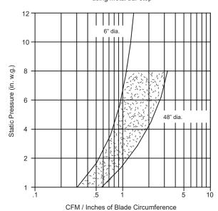
Leakage results shown are based on tests using various damper sizes. The shaded area between the graph lines indicate normal expected leakage range for a standard damper operating conditions and sizes.
